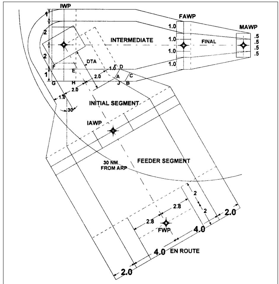
*The segments of a GPS instrument approach from FAA Order 8260.38A. Note the final approach segment primary area is only 0.5 nm either side of centerline, which is closer to ILS tolerances than the typical non-precision approach. Abbreviations: ARP - Airport Reference Point, FWP - Feeder Waypoint, IAWP - Initial Approach Waypoint, IWP - Intermediate Waypoint, FAWP - Final Approach Waypoint, MAWP - Missed Approach Waypoint.*
