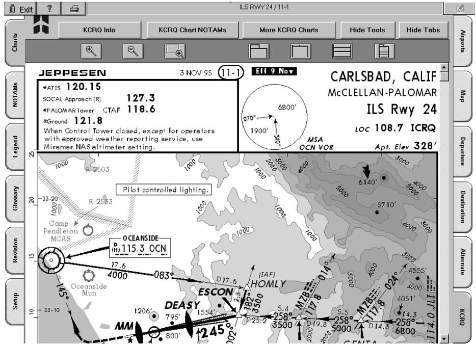
**Figure 1.** JeppView screen showing partial plan view of KCRQ ILS Runway 24. Because the standard PC screen doesn't scale to the approach chart's dimensions, it's necessary to select portions of the chart at a time. On a good PC display, the plan view of any JeppView with color terrain contours is spectacular.
