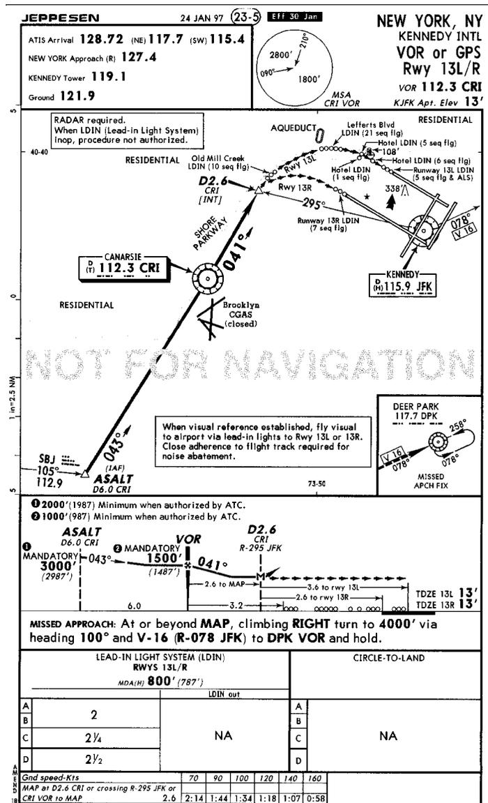
Figure 2. The missed approach points on this procedure are so far from the airport that the result is nothing more than a bad-weather visual approach procedure.
