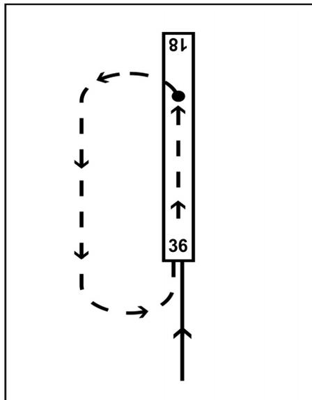
Figure 4. For a circling approach where the electronic final is aligned with the runway, fly down the runway at MDA until it's about to disappear under the nose, then enter the close-in circle-to-land maneuver.
