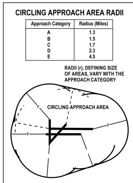
Figure 1. Circling approach protected airspace varies by aircraft category. The HAA must be at least 350 feet for Cat A, 450 feet for B & C, and 550 feet for D & E.
