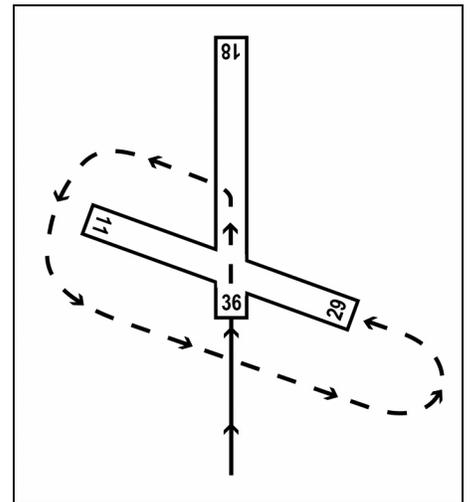
Figure 6. You want to land on Runway 29, but it's too close to break-off and enter left circling. In this situation, fly down the runway until crossing Runway 11/29 and circle to the left in order to keep the runway visible at all times.
