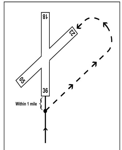
Figure 5. Because the intersection of Runway 23 with the IAP runway is sufficiently down-field, you can break off the electronic final in a manner similar to the "classic" circle-to-land in Figure 2.
