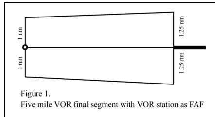
*Figure 1. Because the missed approach point is five miles from the station, there is effectively 14 degrees of VOR error protection.*
