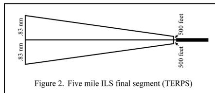
*Figure 2. Old lateral limits of ILS final segment were conservative, but not any more (see Figure 3 below).*
