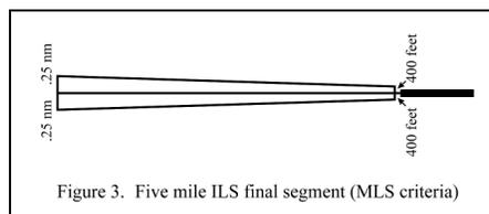
*Figure 3. The lateral limits of the ILS final segment for all new and revised ILS IAPs. Keep that localizer centered folks.*
