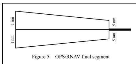
Figure 5. The standalone GPS final approach segment is generous at present, but will probably be drastically reduced once DGPS is in use.
